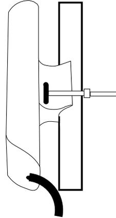
The Bridge is most easily mounted to a pole with a zip-tie, as shown. The Ethernet Cable is connected to the PoE port of the power supply.
