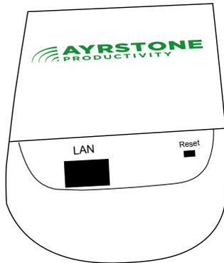
Plug the other end of the Ethernet cable from the "POE" side of the power supply into the port on the Bridge radio - slide in until it clicks in place
