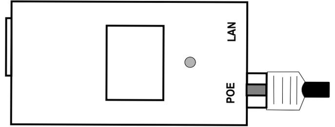
Use another Ethernet cable to connect the LAN port of the power supply to one of the LAN ports on your router.
