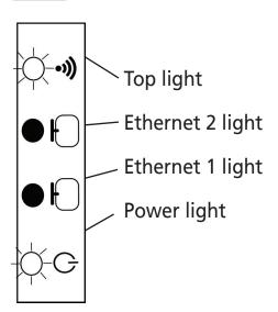
Gateway Hubs have the Power light on steady, and the Top Signal light on steady. One of the Ethernet lights will be blinking.
