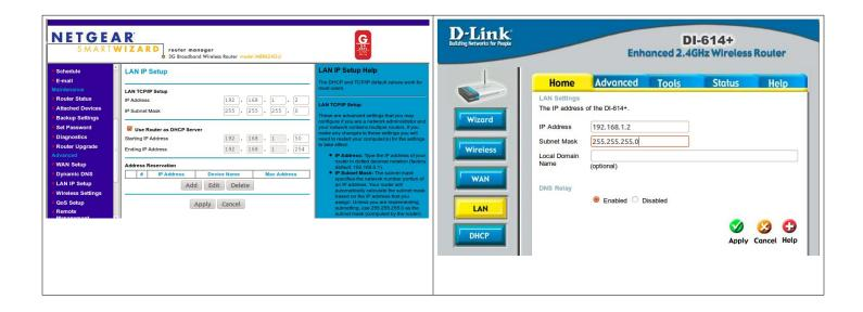
Make sure that the router has an IP address different from the main router but in the same subnetwork as the main router. Because my main router is at 192.168.1.1, I set the address for this "auxiliary" router at 192.168.1.2. Note that the first three numbers are the same, but the third number is different.
