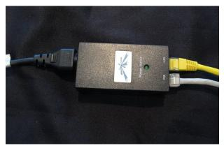
Make sure that you can plug a computer into the LAN port on the Power supply and access the Internet on that computer.
