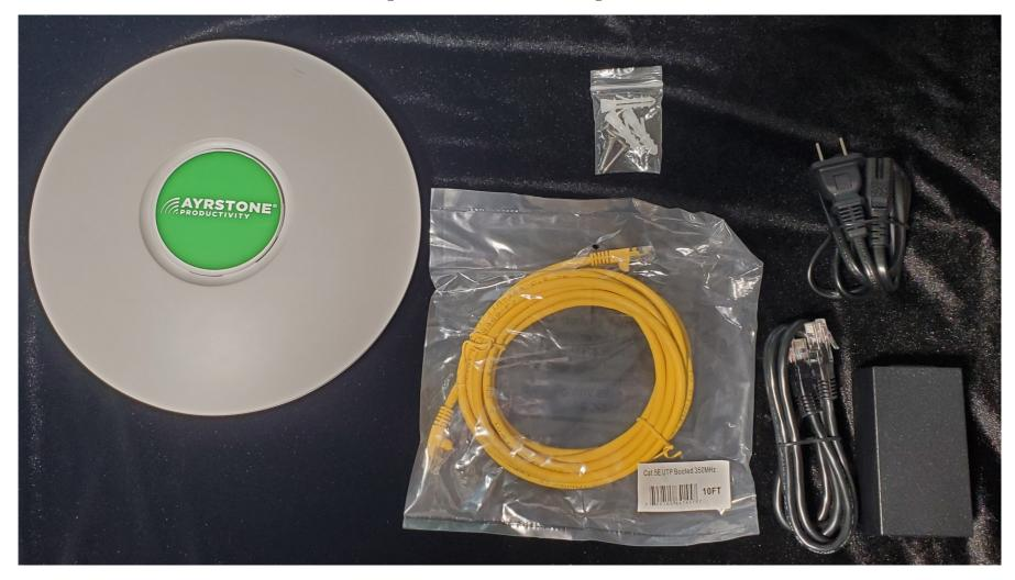
From left to right – IndoorHub, long Ethernet cable, screws, short ethernet cable, power cord, power supply
