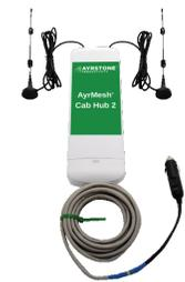
The AyrMesh Cab Hub2 is a special Hub that is used on farm equipment - tractors, sprayers, combines, even trucks or UTVs - to provide connectivity for devices in and around those machines. It works just like any other Hub, but connects to the in-cab power and includes special antennas for use on vehicles. It communicates with all the Hubs on your network to keep you connected.
